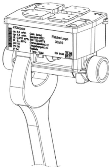
Make sure the flow sensor is installed sufficiently far away from possible sources of electromagnetic interference (switches, electric motors, fluorescent lamps, etc.). At threshold connection a tool to hold the meter at the mounting process must be used.
